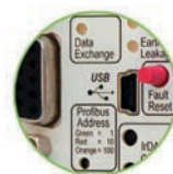
IRDA & USB Communication & Profibus address indication.
